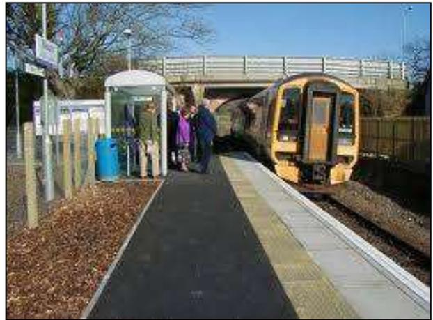
**NORTHERN RAIL** suggested their eco-shelter at Maryport, Cumbria. This is a timber shelter made by Littlethorpe of Leicester (FSC certified supplier). As shown in the picture (*right*), it has solar panels on the roof and uses glass rather than polycarbon. Advice suggests that it is also carbon neutral.
